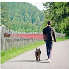
Adjust the installation height and the detection angle to avoid the small animals to activate the sensor.
